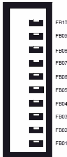
Feature Buttons (FB) are numbered from the bottom up as shown here.
